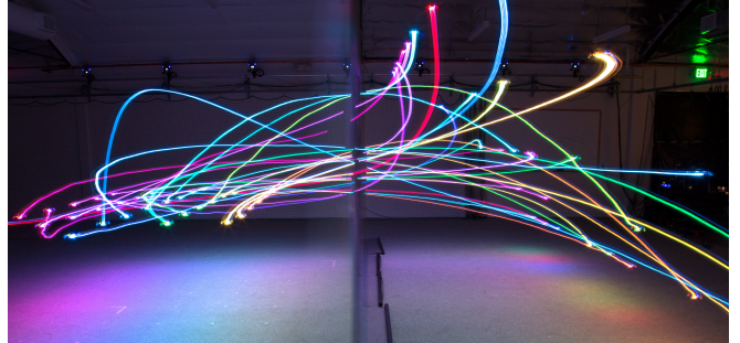
Fig. 1. Long exposure of 32 Crazyflie nano-quadrotors flying through a wall with windows, viewed from the edge of the wall.
