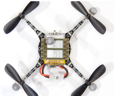
Fig. 1. The Crazyflie 2.0 miniature quadcopter with four motion-capture markers, LED expansion board (not visible), and battery.
