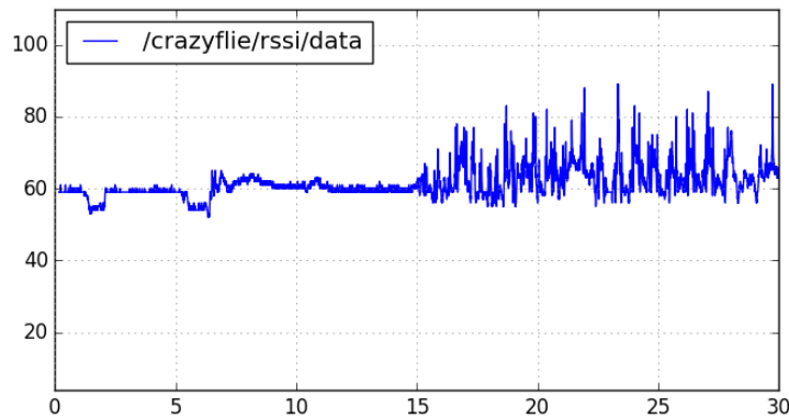
Fig. 6. Output of rqt_plot showing the radio signal strength indicator. The first 15 s show a good signal, while the second half shows higher values and noise caused by interference.
