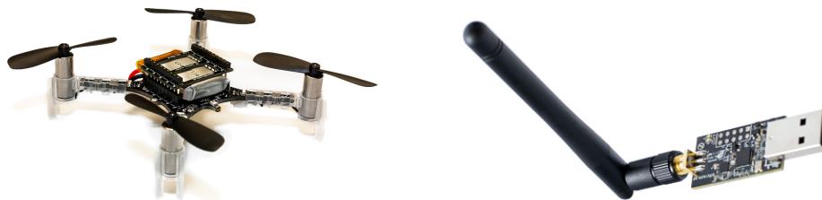
Fig. 1. Our target platform Bitcraze Crazyflie 2.0 quadcopter (left), which can be controlled from a PC using a custom USB dongle called Crazyradio PA (right). Image credit: Bitcraze AB.
