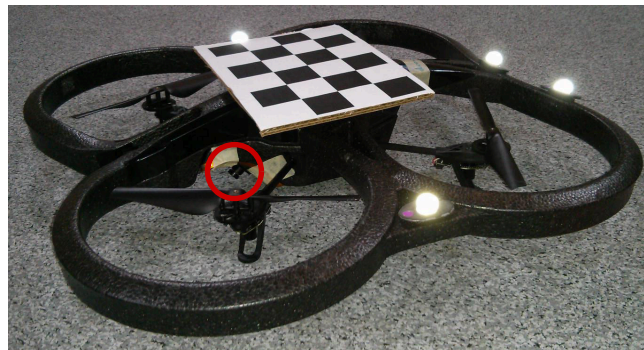
Figure 9. The AR.Drones are equipped with a checkerboard and Vicon markers for relative sensing and ground truth poses, respectively. The forward-looking camera is tilted 45° downwards (highlighted by a red circle) to track the target and robots on lower levels of the sensing topology.
