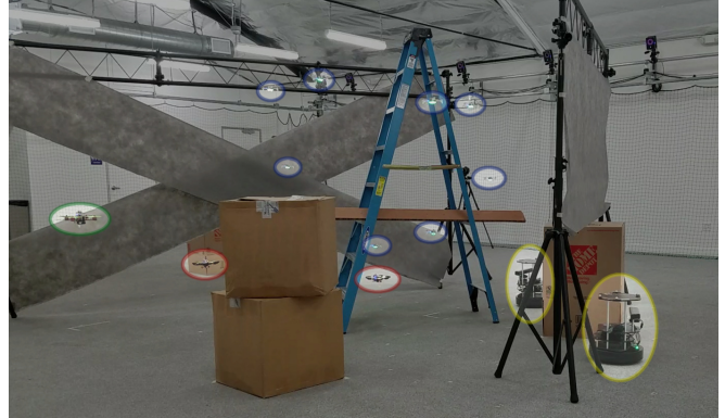
Fig. 1. Heterogeneous robot team with ten small UAVs (blue, only eight visible), two medium UAVs (red), one large UAV (green), and two ground robots (yellow). The robots have to navigate through a cluttered environment, avoiding obstacles and taking asymmetric inter-robot constraints into account.
